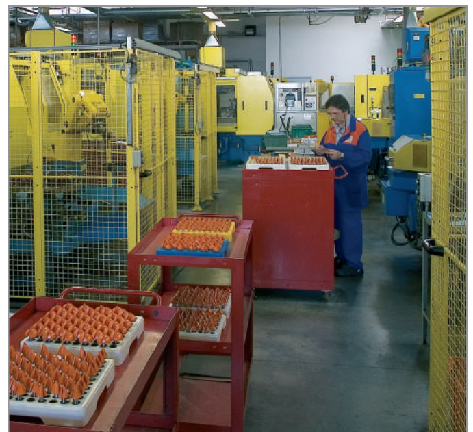
Loading the automated multi-axis CNC sharpening machines.
