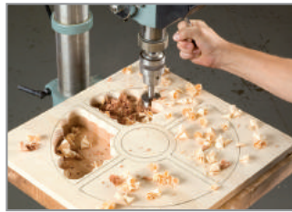
Rough out the interior using a drill press and a 50,8mm Forstner bit.
